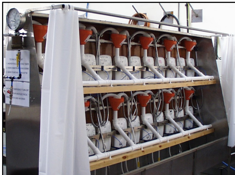
Product evaluation rig for domestic shower units (temporary facility)
