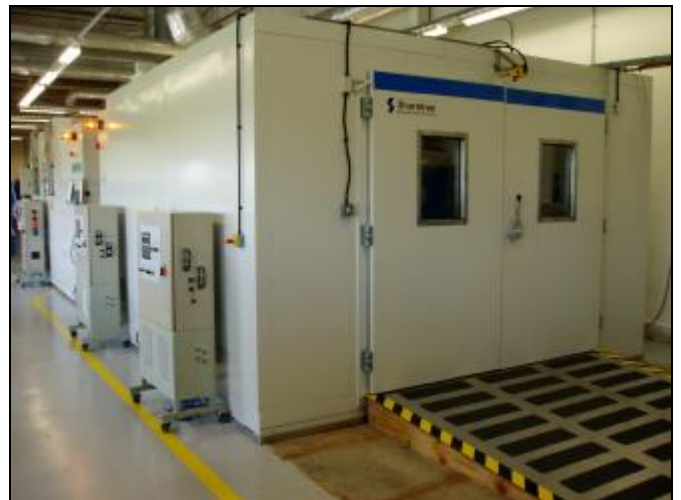
Large walk-in chambers for Automotive testing
