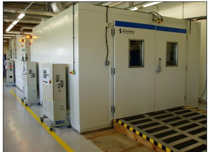
*Large walk-in chambers for testing of Automotive products.*
